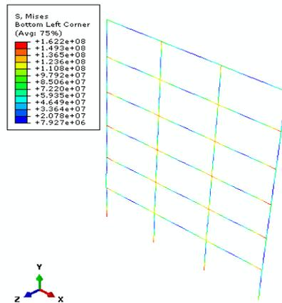
Figure 9. Von Mises Stress in M6 model
