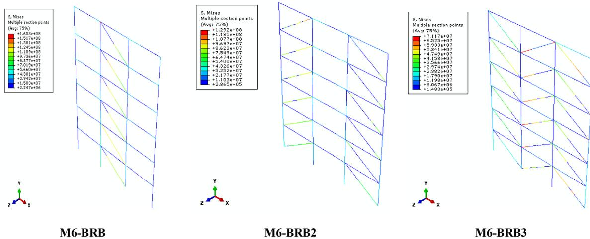
Figure 12. Von Mises stress in six stories model
