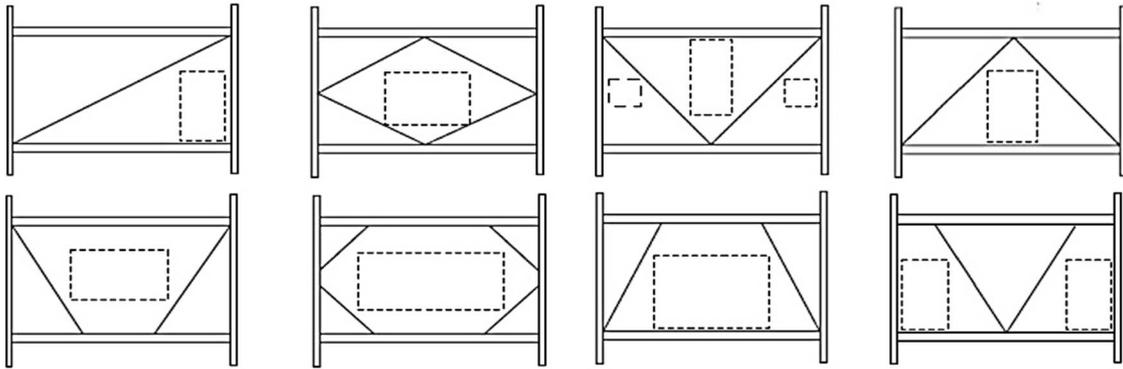
Figure 1. Examples of converge and divergent braces [12]
