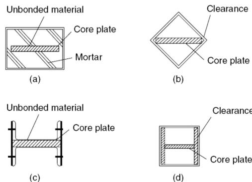
Figure 4. Enclosure mechanism of the core with mortar [10]
