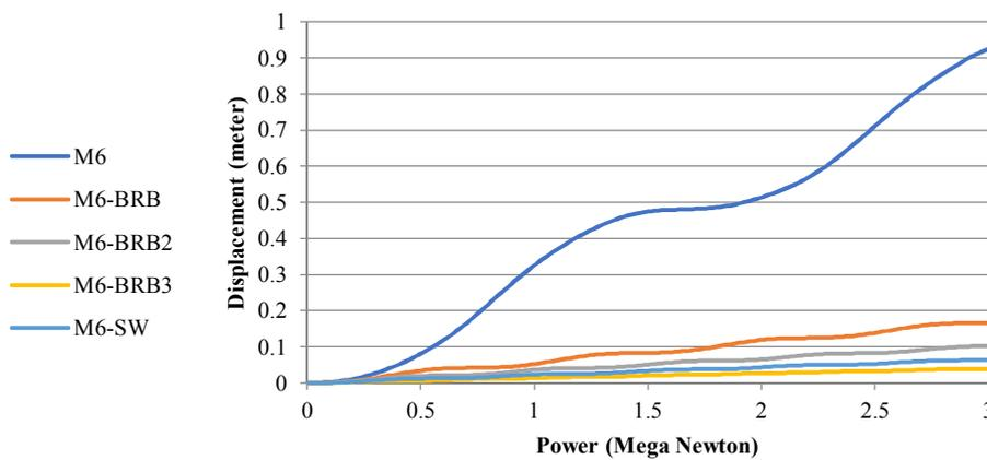
Figure 15. Power-displacement curve of 6-story models
