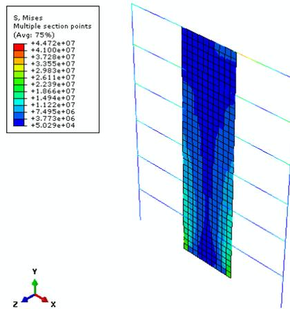
Figure 14. Von Mises stress in M6-SW model
