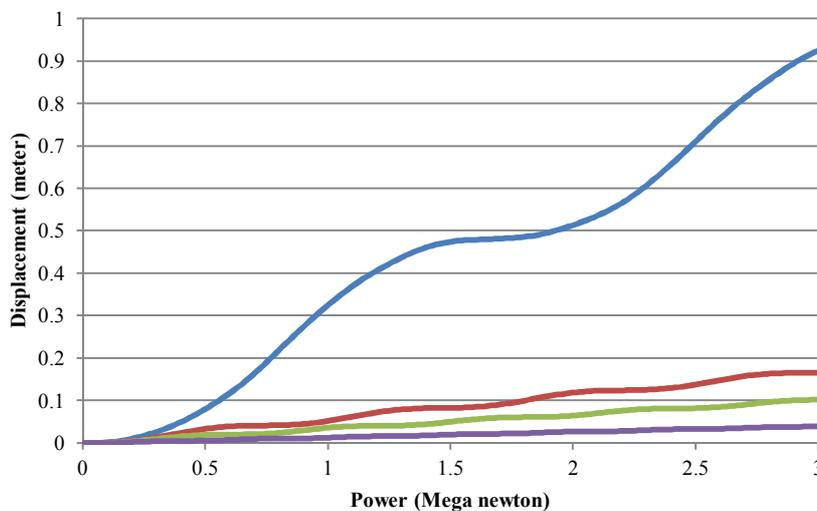
Figure 13. Power-displacement curve of 6-story models with BRB brace
