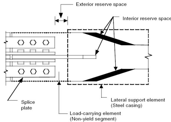
Figure 3. Empty space to prevent the contact between steel plate and mortar [10]
