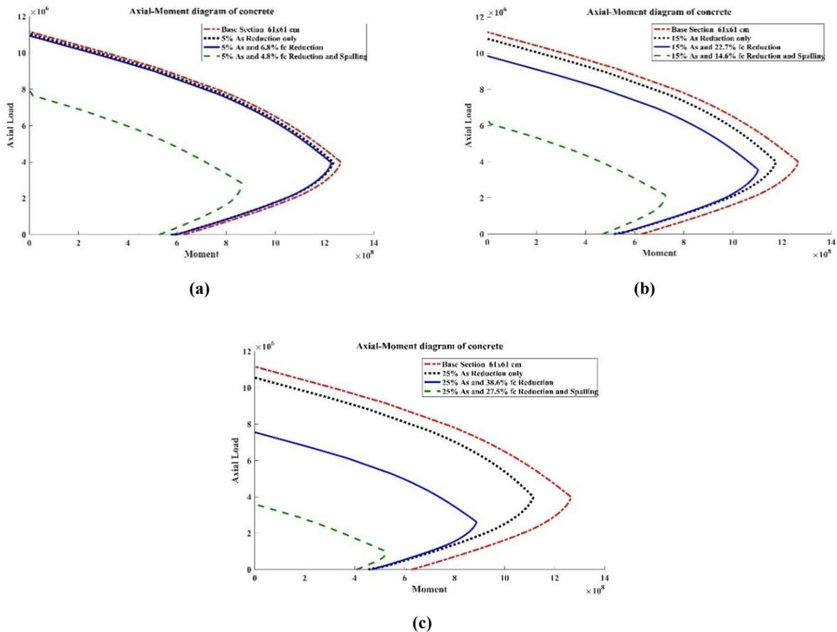
**Figure 8: Interaction Cross-Sectional Curve with 0.016 (12F25) under a) 5% corrosion b) 15 %corrosion c) 25 % corrosion**
