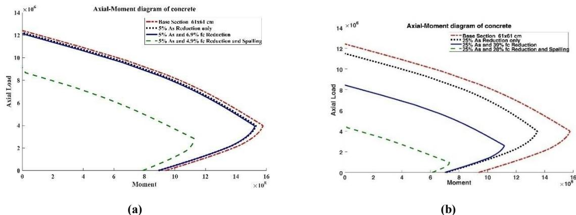
**Figure 7. Interaction Curve of the Cross Section with a Yield Stress of 5000 MPa under a) 5% corrosion b) 25% corrosion**
