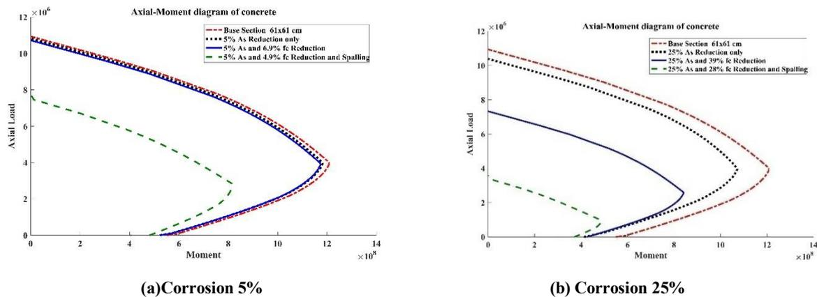
**Figure 6. Interaction Curve of the Cross Section with a Yield Stress of 3000 MPa under Corrosion**
