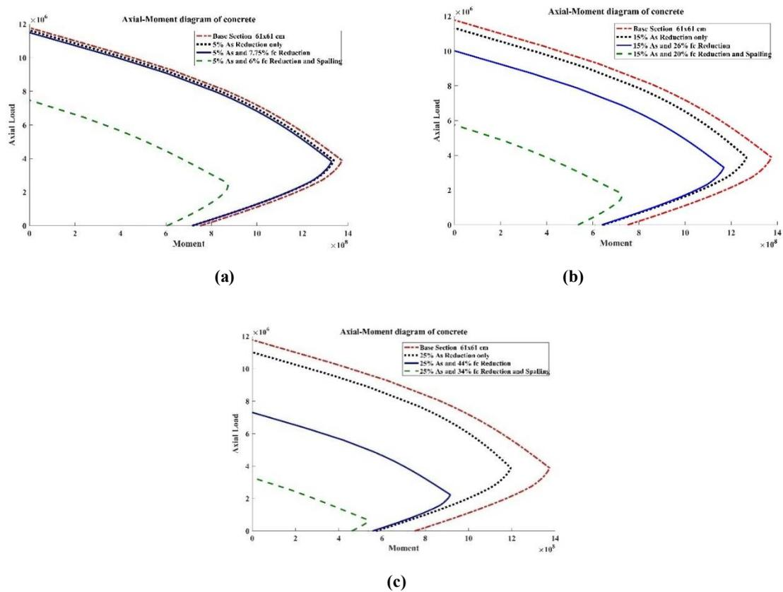
Figure 5. Interaction Curve of the Cross Section with a Coating of 7 cm under a) 5% Corrosion b) 15% Corrosion c) 25% Corrosion
