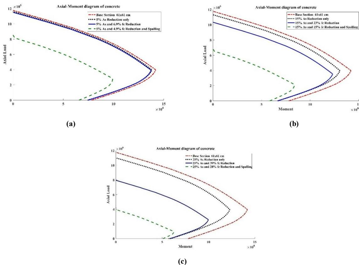
Figure 2. Interaction of the Primary Section Curve under a) 5% Corrosion b) 15% Corrosion c) 25% Corrosion
