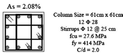
Figure 1. Base Section Details [26]
