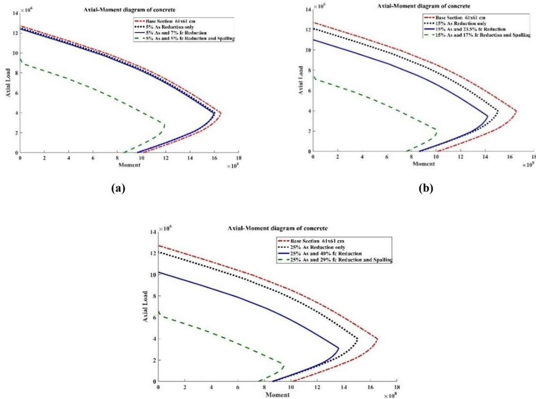
Figure 9. Interaction Curve with Cross-Section Ratio 0.026 (12F32) under a) 5% Corrosion b) 15% Corrosion c) 25% Corrosion
