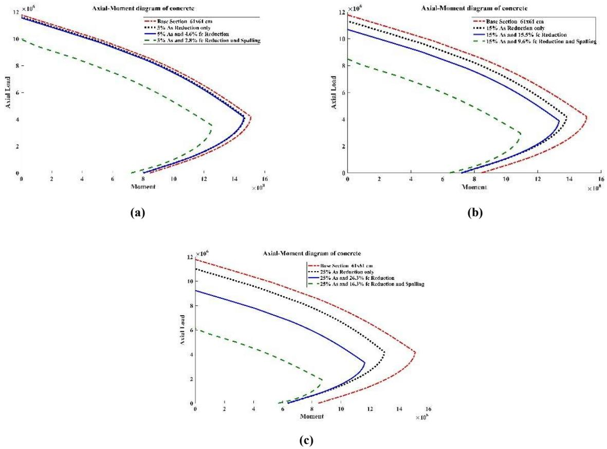
Figure 4. Interaction Curve with a Coating of 2.8 cm under a) 5% Corrosion b) 15% Corrosion c) 25% Corrosion
