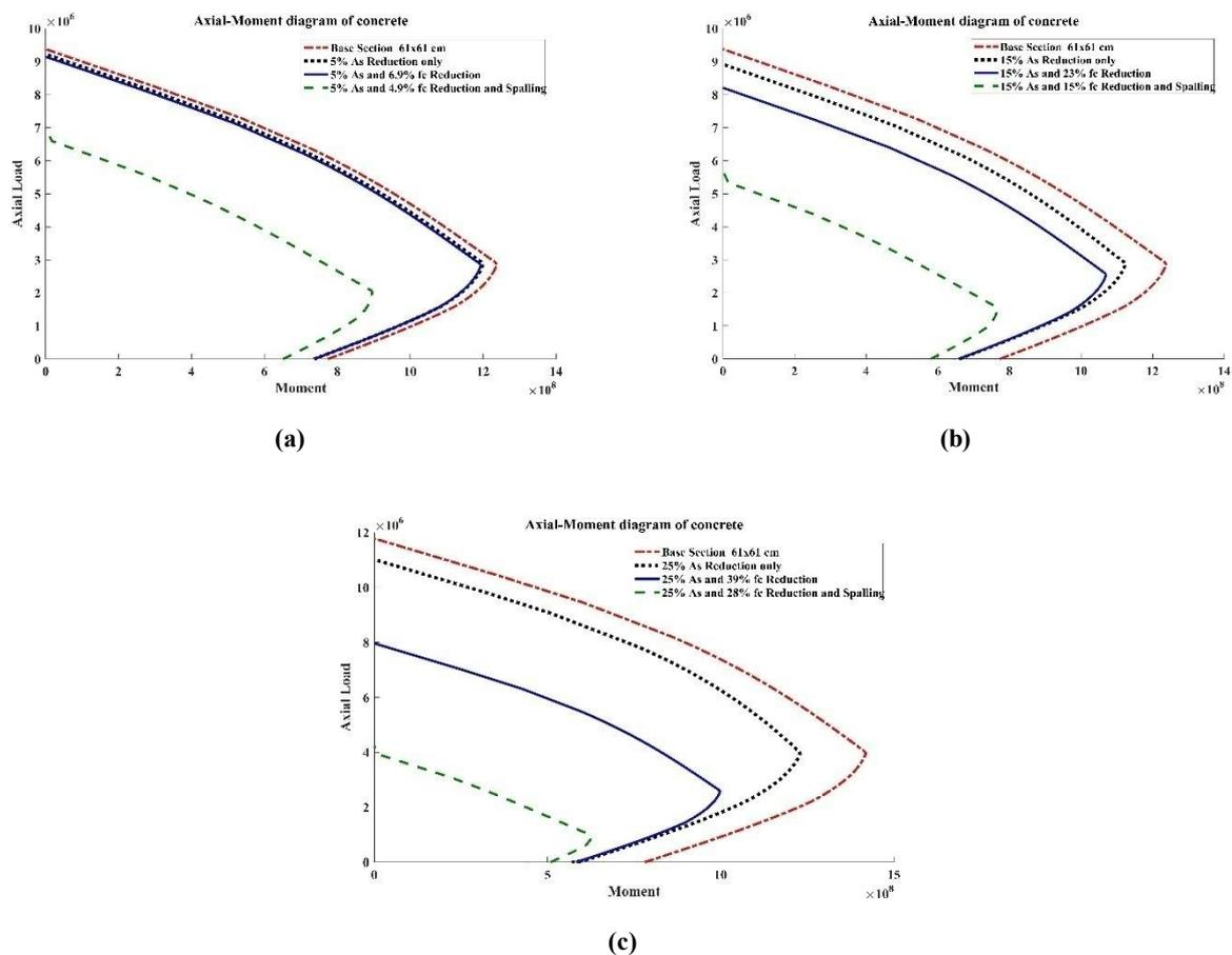
**Figure 3. Interaction of the Primary Section Curve with 20 MPa concrete under a) 5% Corrosion b) 15% Corrosion c) 25%Corrosion**
