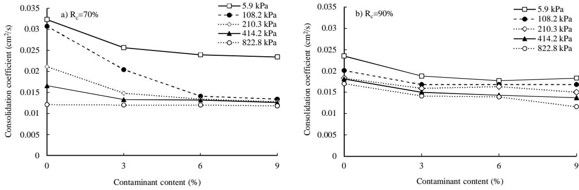
Figure 7. Variation of consolidation coefficient for kaolinite contaminated with kerosene
