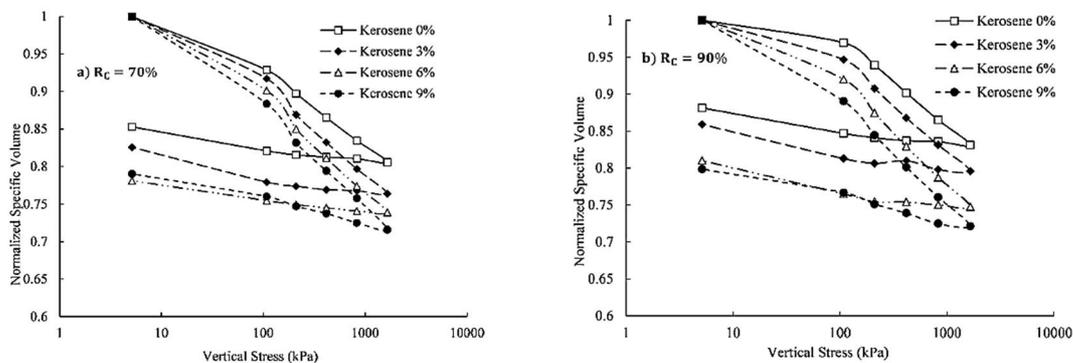
Figure 4. Consolidation test results on kaolinite contaminated with kerosene
