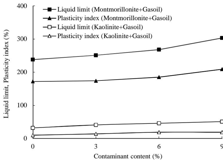
Figure 2. Liquid limit and plasticity index of montmorillonite and kaolinite contaminated with gasoil
