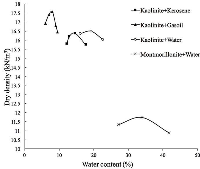
Figure 3. Results of standard Proctor tests on kaolinite and montmorillonite including water, kerosene and gasoil as pore fluid
