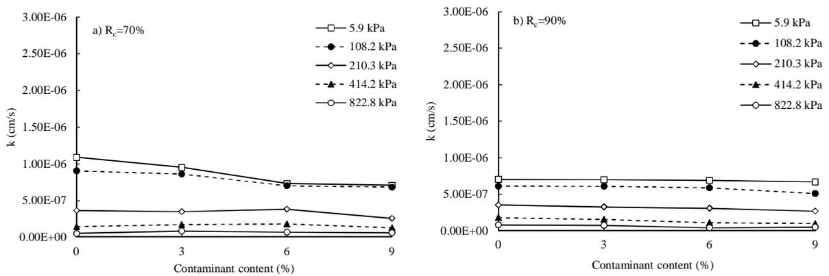
Figure 11. Variation of permeability coefficient for kaolinite contaminated with gasoil
