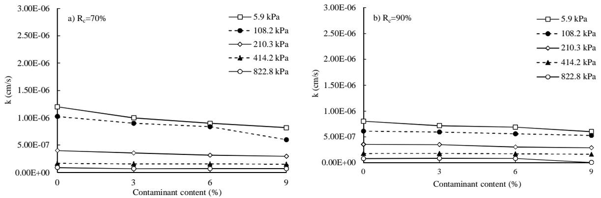
Figure 10. Variation of permeability coefficient for kaolinite contaminated with kerosene
