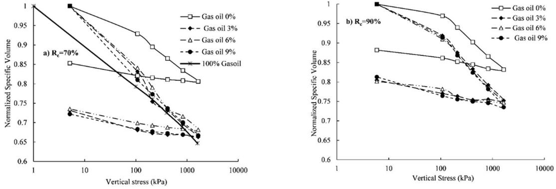
Figure 5. Consolidation test results on kaolinite contaminated with gasoil
