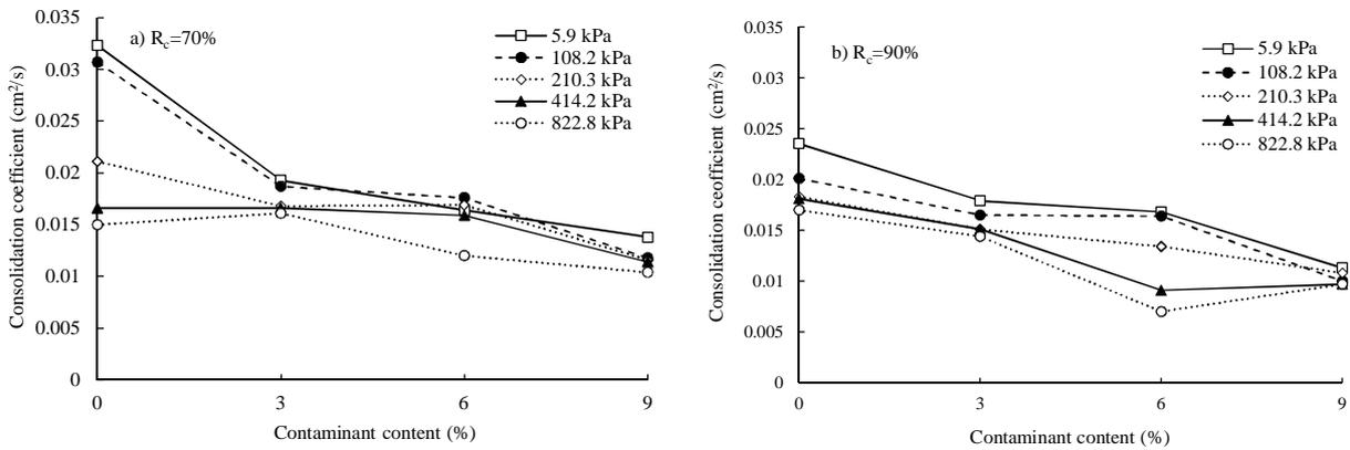
Figure 8. Variation of consolidation coefficient for kaolinite contaminated with gasoil
