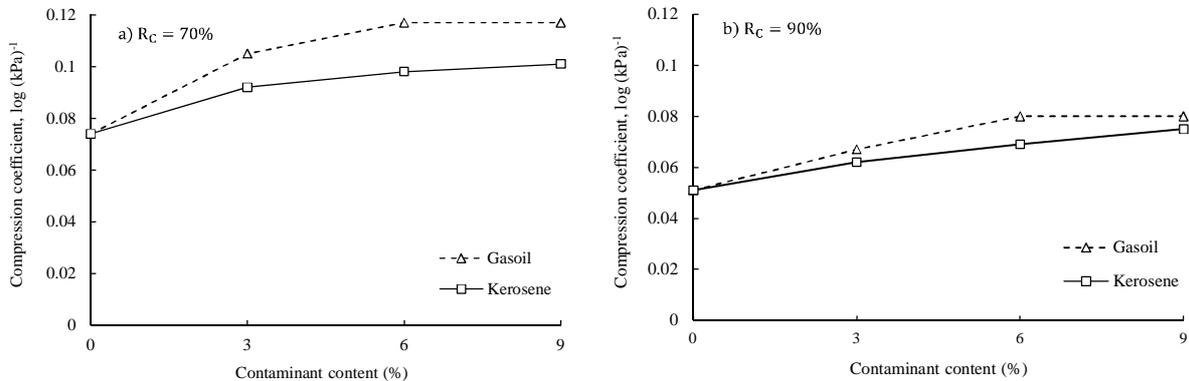
Figure 6. Variation of compression coefficient of kaolinite contaminated with kerosene and gasoil
