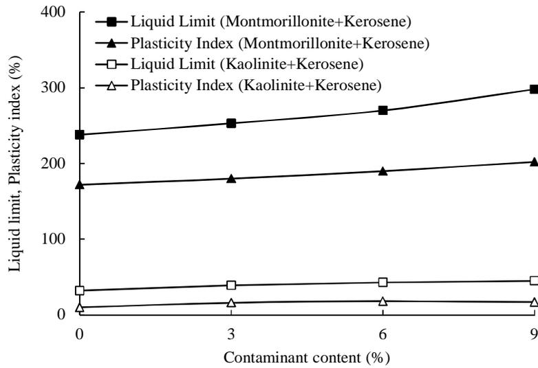
Figure 1. Liquid limit and plasticity index of montmorillonite and kaolinite contaminated with kerosene
