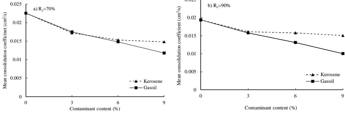
Figure 9. Variations of the mean consolidation coefficients obtained in different surcharge pressures with contaminant content.
